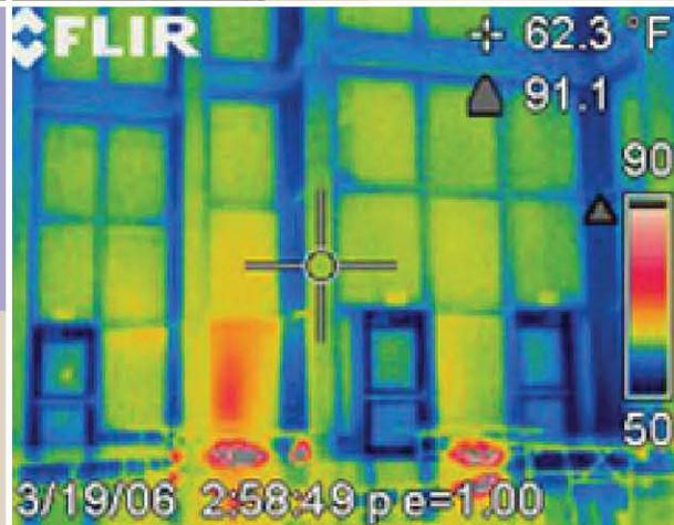
A thermal imaging scan (above) shows superior insulation values for the triple glazed curtain wall (see picture, left) in the commons area.
